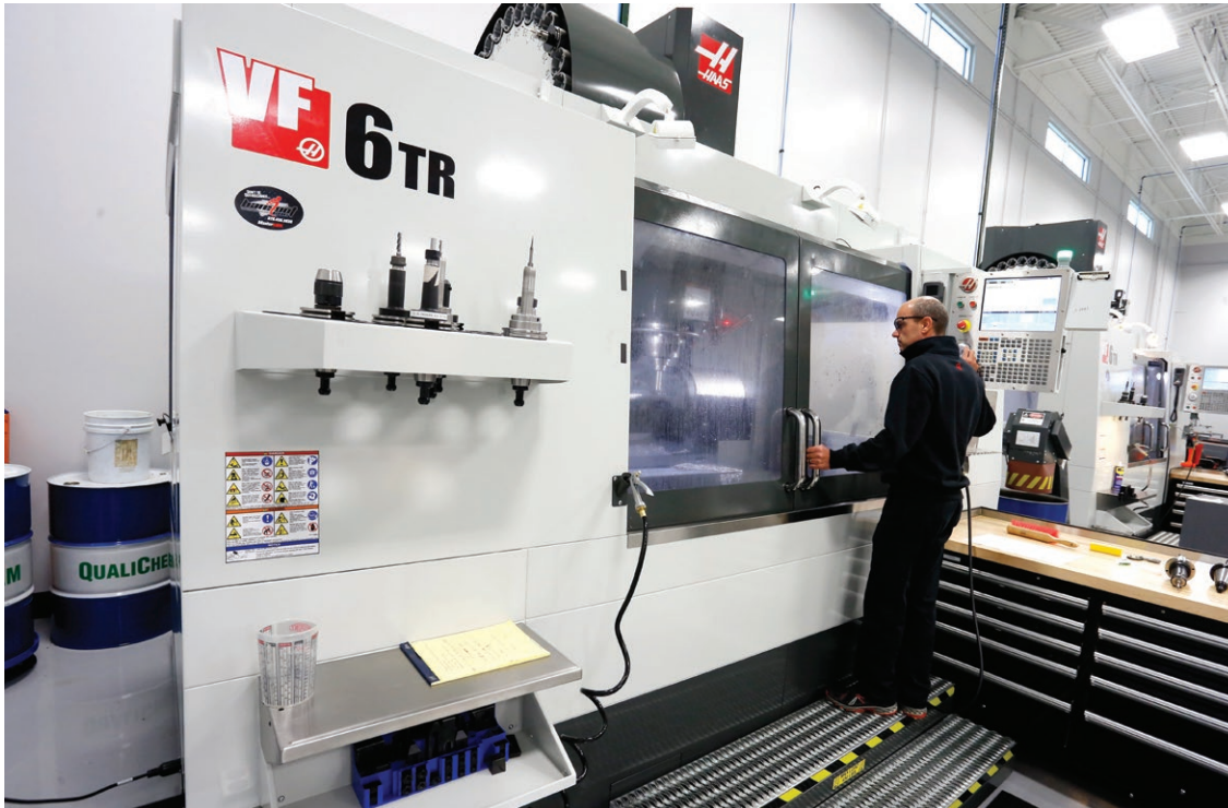
An employee works on a Haas CNC milling machine at the new Kannapolis headquarters.
