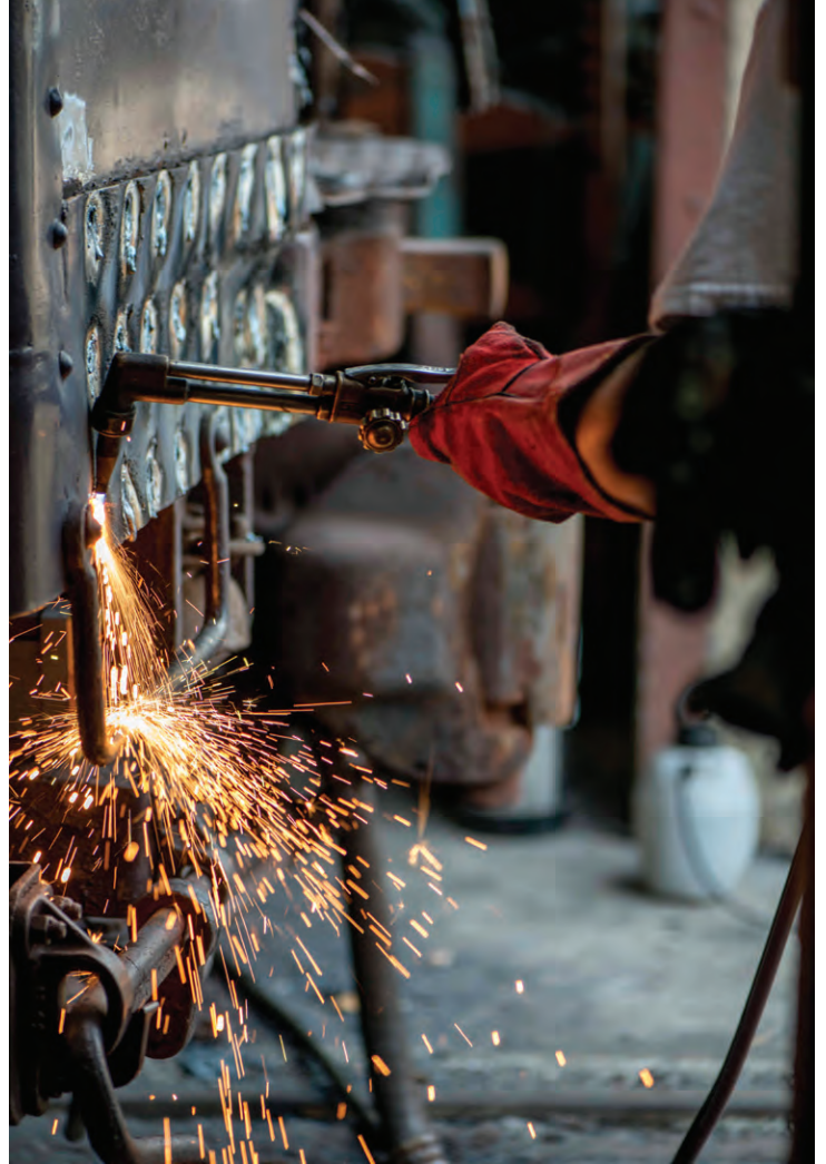
Above: Volunteer conductor Charlie Davis speaks to visitors. Right: Vincent Owens uses an acetylene torch to cut the rivets off of a panel on the back of a coach car under restoration. Below: The Back Shop is a popular place for events. Left: A 1935 Ford convertible Highway Patrol car.
