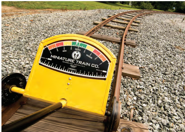
Top: The miniature train engine weighs about a ton. Above: A look at the engine's instrument panel. Below: The hand-pushed gauge measures the width of the track. Left: The Deals approach the crossing sign where their train crosses the driveway.
