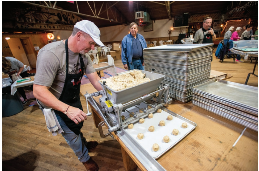
Jeff Smith uses a new addition to the cookie factory, a Kook-E-King cookie depositor.
