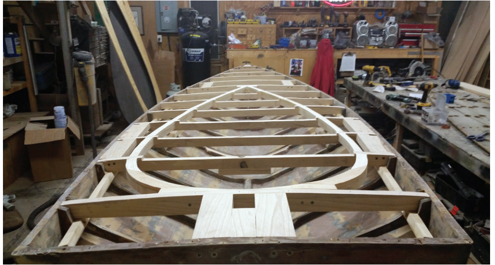
Above: Some of the extensive wooden infrastructure in the 1870 scull boat. — Photo courtesy of Brad Taylor. Below: Brad Taylor used pieces of tigerwood, walnut, padauk and ash to make this endgrain cutting board. — Photo courtesy of Compass Woodworks Co.
