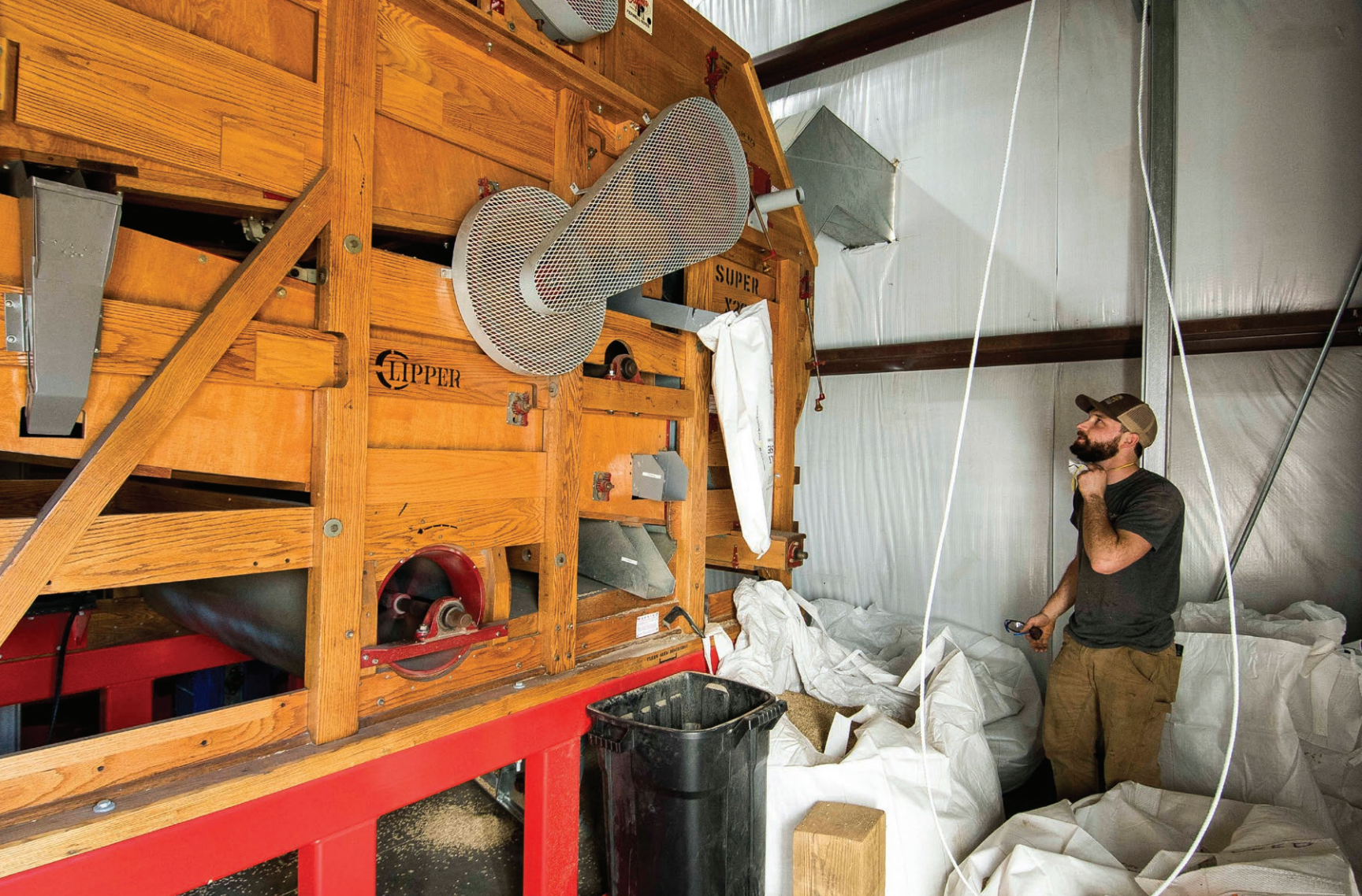
Mark Van Wagenberg operates the Clipper Super X 298D cleaner, one of the first steps in the malting process.
