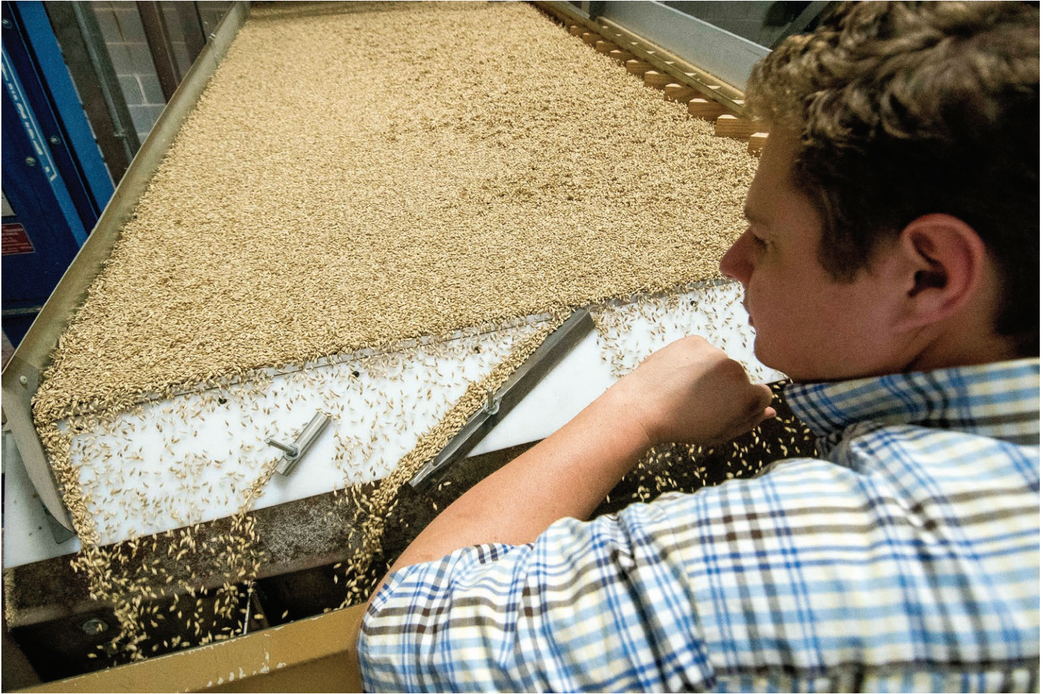
Aaron Goss inspects the barley kernels that travel across the top of the Oliver 240 gravity table — a step before the steeping process.
