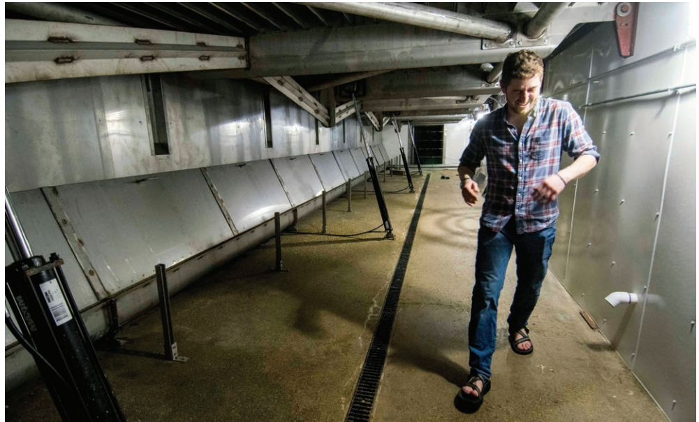
Steve Bauk makes his way quickly through the lower level of the Saladin box during a day when the kiln temperature was about 130 degrees. A hinged floor drops barley on the upper level to this part of the kiln from where it is conveyed out.
