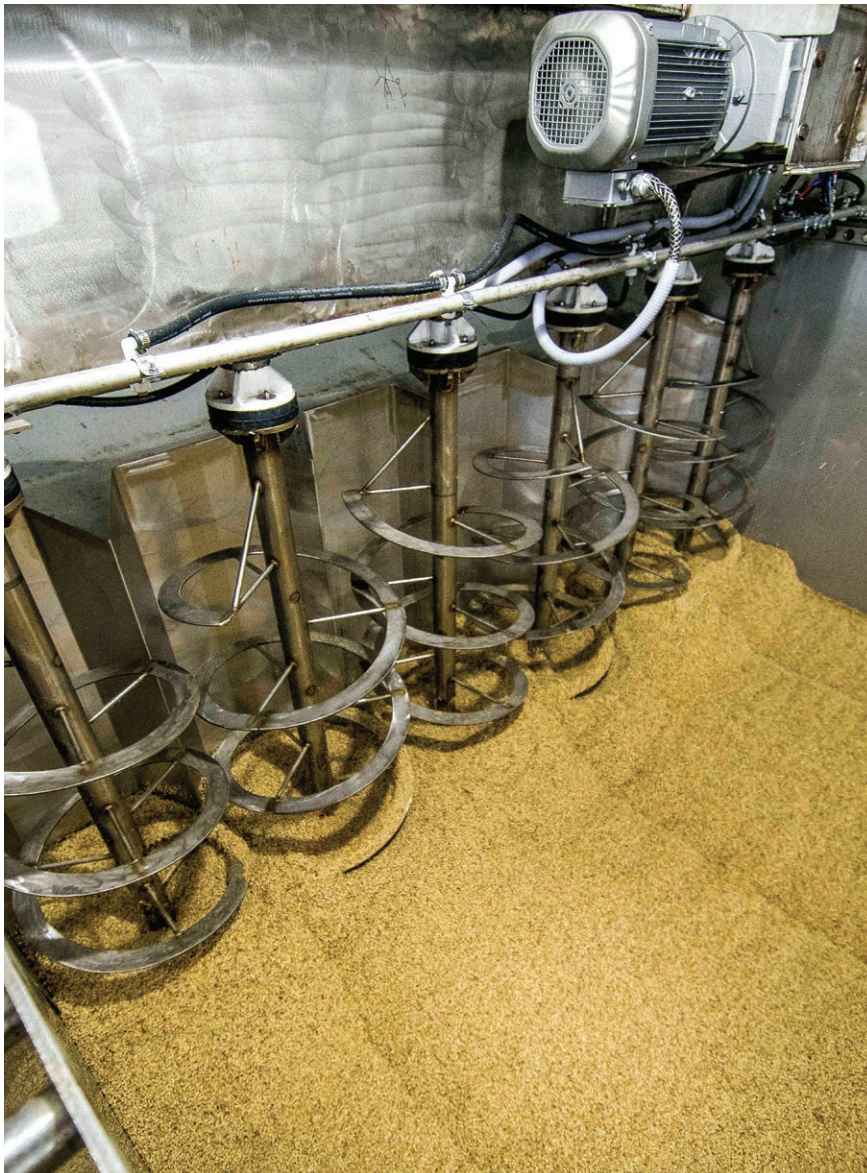
Inside the two-level box, the barley continues to germinate while being constantly turned.
