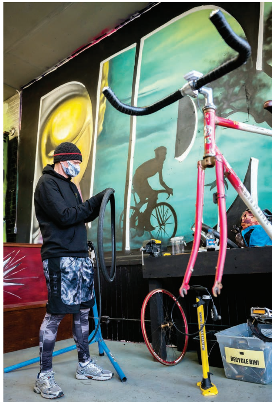
Volunteer and bike mechanic Tim Faucette works on getting a fresh inner tube and tire onto a bicycle wheel during shop hours.
