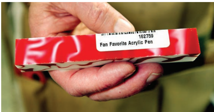
The acrylic blanks used for the pen bodies comes in all sorts of colors like this red and white with marbled coloring inside.
