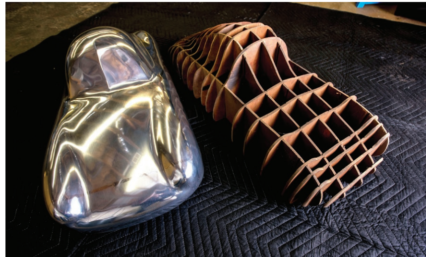
Miller created a model of the car, left, using a wooden buck, right.
