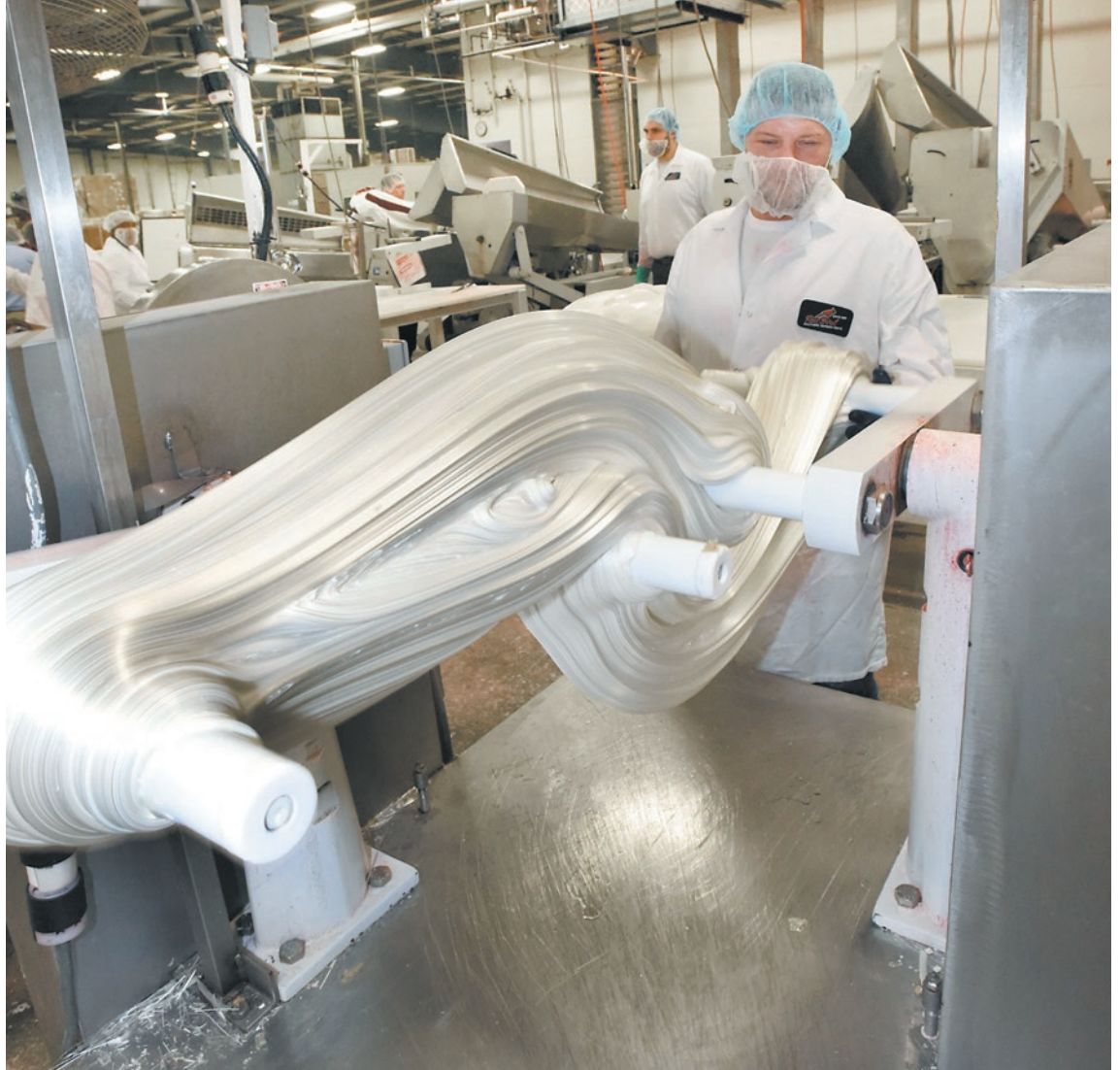
Right: A worker runs a pulling machine for a 100-pound batch of candy, making it glossy.
